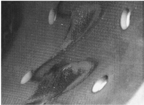
Fig. 10 Inner side of the SiC/SiC flame tube after 30 h of engine operation
